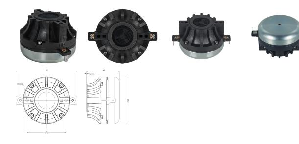
Very Compact 69 mm diameter 80 W\* continuous program power capacity 1" horn throat diameter 44 mm (1.7 in) aluminium voice coil HT Polymer diaphragm 1000 - 18000 Hz response 109 dB sensitivity Small heat sink required for full power application
