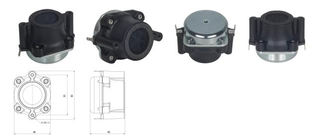
Ultra Compact 48mm diameter 40 W continuous program power capacity 1" horn throat diameter 36 mm (1.4 in) aluminium voice coil HT Polymer diaphragm 1000 - 17000 Hz response 108 dB sensitivity
